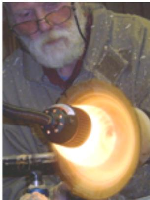
but he left the chucking spigot on, so that the bowl could be re-chucked for finishing when it had dried out over the next few weeks. At this point his demonstration concluded, and he left the almost complete piece for somebody else to finish off.
