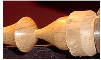
shoulders of the figurine turned and finished as before. It only remained to make the last offset, and the head was turned and mostly finished. Although this is not on the crib sheet, it might be
